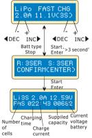
The value on the left side of the second lines sets the charge current. The value on the right side of the second lines sets the battery pack's voltage. After setting current and voltage, press STAR/ENTER for more than 3 seconds to start the process.
