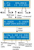
The left side of the first line shows the type of battery you choose. The value on the left of the second line of the charger is current user set, After setting the current and voltage, press START/ENTER key for more than 3 seconds to start the process.(charge current: 0.1-5.0A. voltage: 3.7-22.2V).
